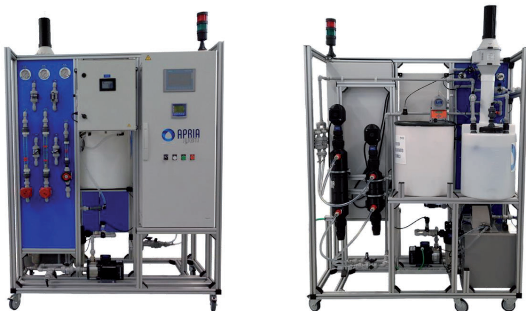
Figura 3-4. Planta piloto Photobench LED275-0.8/LED365-16/450-16a (APRIA Systems): vista frontal y posterior.
